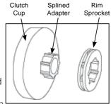
sprocket. When the rim sprocket wears out, it is the only part that needs to be replaced. The clutch cup with splined adapter is a wear item that needs replacement after 3 to 5 rim sprockets have been used.
